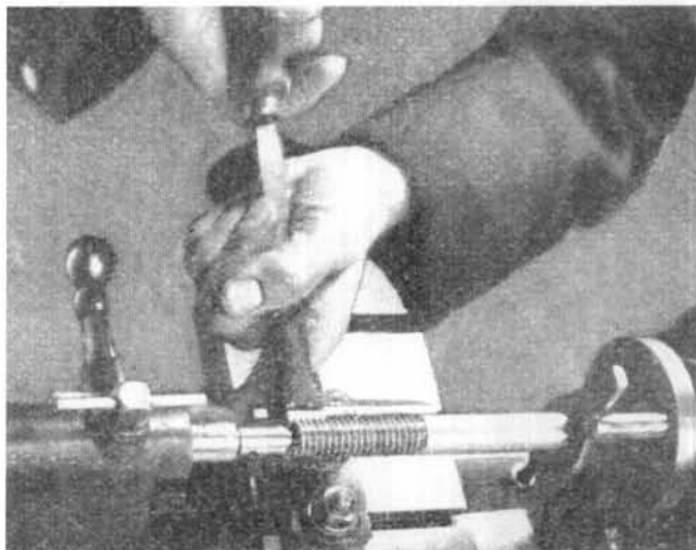
hand chasing an external thread on steel with a treadle powered lathe between centres
